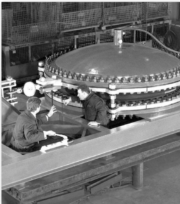
Figure 3. Expansion Joint Stiffness Testing
