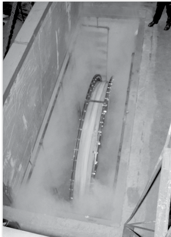
Introduction of swirling steam from multiple jets assures uniform heat distribution and rubber curing. Photo shows pit prior to closing 10" 9600 lb gasketed concrete cover.
