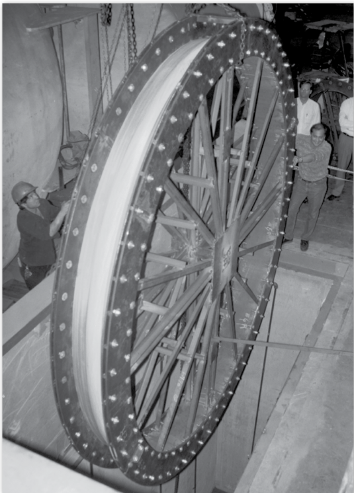
Lowering of 145" ID Expansion Joint into concrete steam curing pit. Weight with mandrel is 6000 lb.
